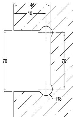
MOUSE EAR CUT-OUT WITH PIN RETAINED
