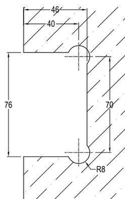
MOUSE EAR CUT-OUT WITH PIN RETAINED
